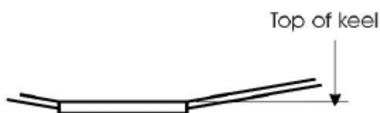
a) Timber deck with rise of keel and deck camber
