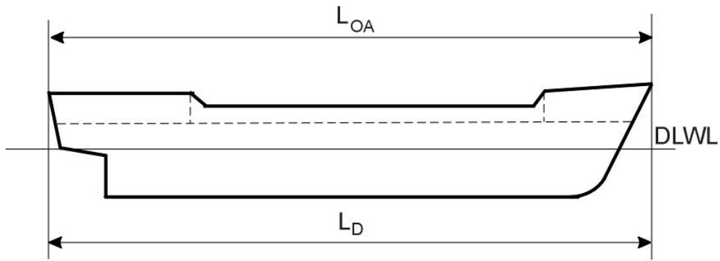
d) Raised fo'c'sle and poop deck
