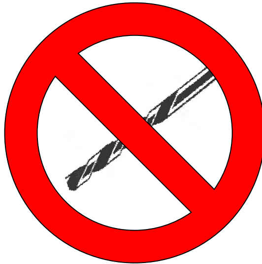
Figure G.1 — Do not penetrate bulkhead sign
