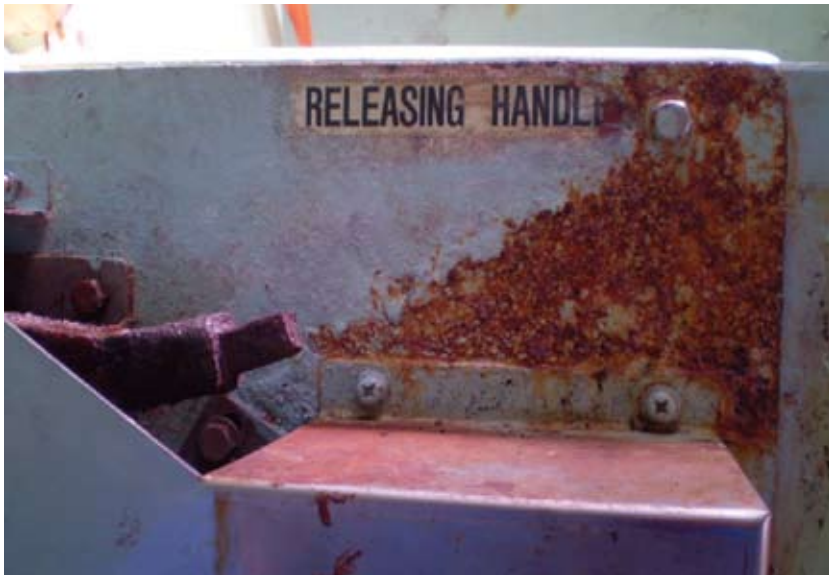
Lifeboat release handle missing
