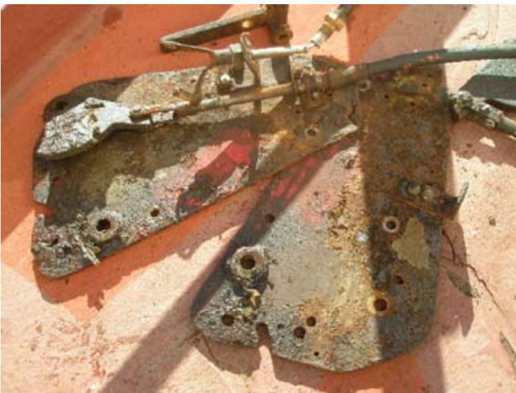
Condition of lifeboat release and interlock arrangements
