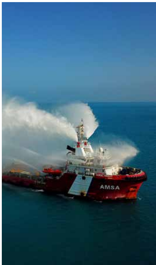
Coral Knight using its FiFi system
