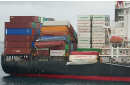
Containers on the YM Efficiency toppled over and falling into the sea. Image supplied.
