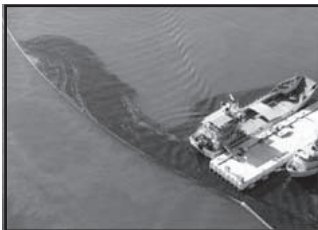
Oil contained in booms in Sydney Harbour during the response to the spill from the Laura D'Amato .
