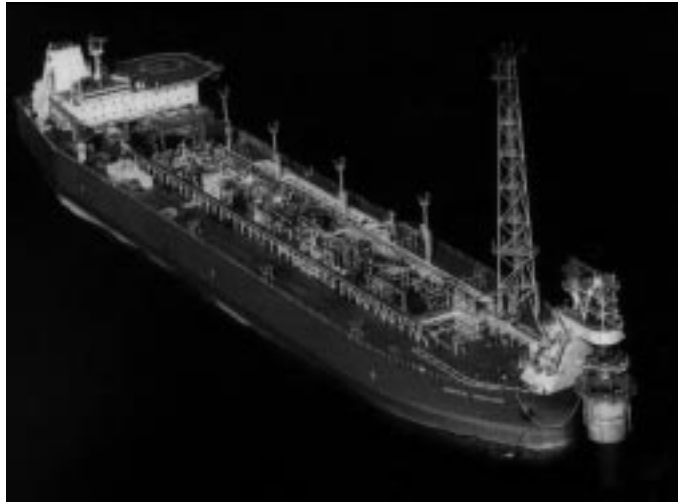
Photo 11. Griffin Venturer Floating Production and Storage Operation (BHP Petroleum)
