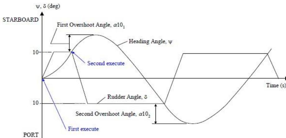
*"Second execute" is to be made when the vessel reaches the specified heading change. However, as reversing of the rudder also takes finite time, the actual change in heading may be different from the specified value.*
