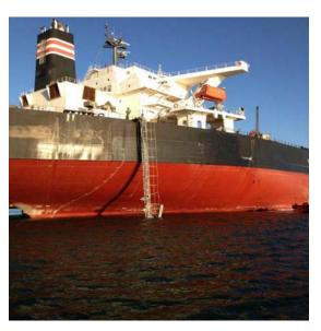
AMSA is aware that arrangements at some berths in Australia prevent accommodation ladders being safely landed on the wharf edge. In such situations it is a common practice to suspend the ship's accommodation ladder at the ship's side with a short brow or gangway fitted to the lower accommodation ladder platform to bridge the gap between the ship and wharf edge.
