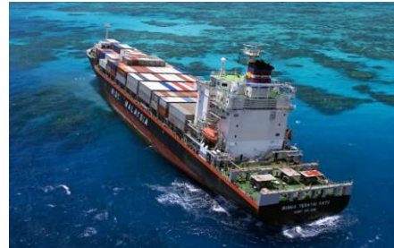
Bunga Teratai Satu, Sudbury Reef, November 2000 failed to make a planned alteration of course and ran aground at 20 knots
