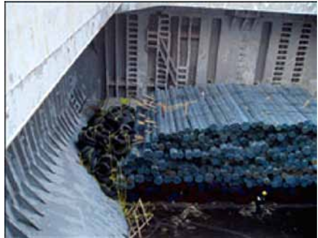
Cargo in hold ends limiting access to hold ladders from the centre of cargo hold
