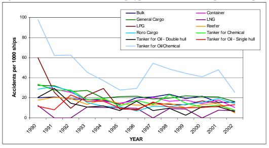
Figure 5-8 Accident trend broken down on ship types, serious acc. pr 1000 ships, 1990-2002
