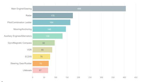
Figure 25. Top 10 most frequently occurring equipment failures reported (2019)
