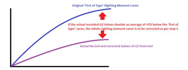
Figure – Showing 'first of type' righting moment curve corrected using 'as built' calculated GZ deviations
