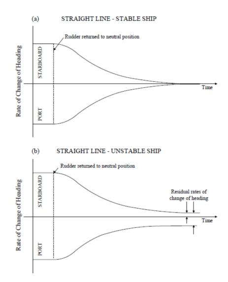
The following trials should be undertaken to identify any un-desirable characteristics of the vessel:
