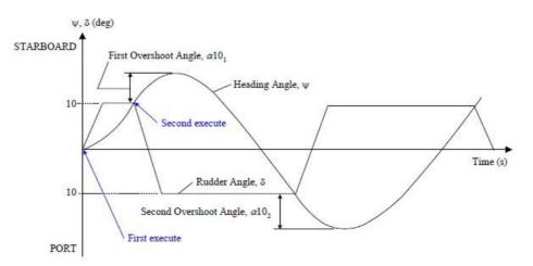
"Second execute" is to be made when the vessel reaches the specified heading change. However, as reversing of the rudder also takes finite time, the actual change in heading may be different from the specified value.
