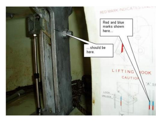
2. Morse Cable corroded and outer sheath detached leaving flexible core of cable holding mechanism in place.
