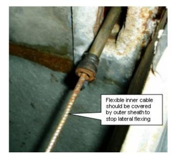
3. Release mechanism (on falls and painter) seized and morse cable corroded
