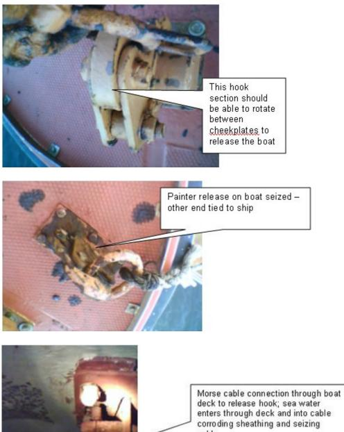
deck to release hook; sea water enters through deck and into cable corroding sheathing and seizing cable
