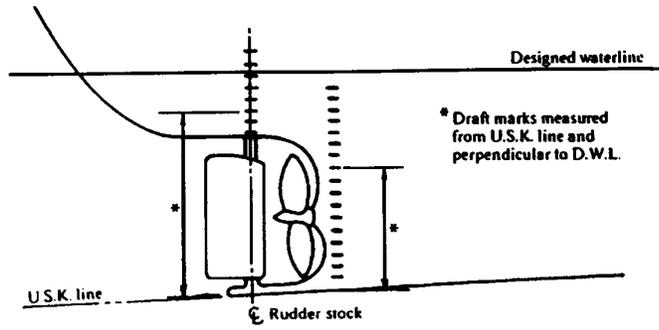
Figure 10 RAKED KEEL – VESSEL WITHOUT A STERN POST
