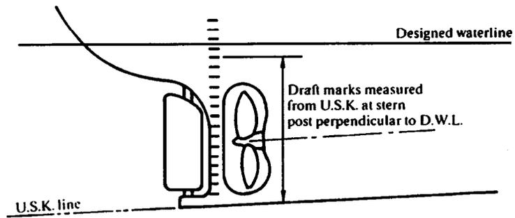
Figure 9 RAKED KEEL — VESSEL WITH A STERN POST
