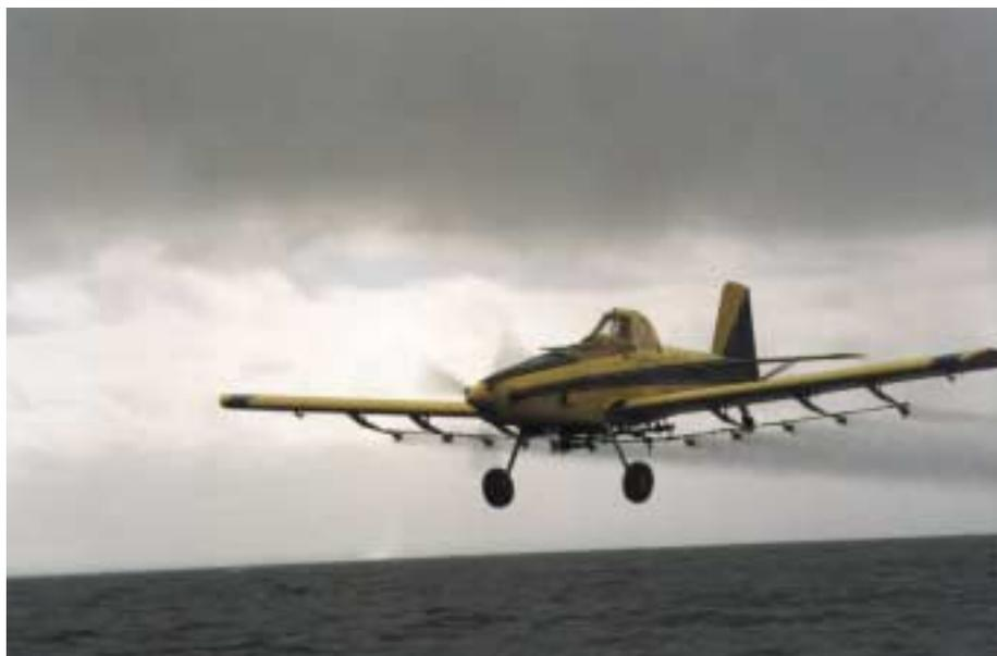
*An Air Tractor used in dispersant application operations*
