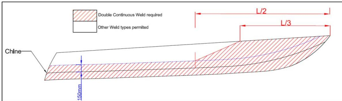
Figure 2: Defined area of double continuous welding (vessel without pronounced Bow Chine)
