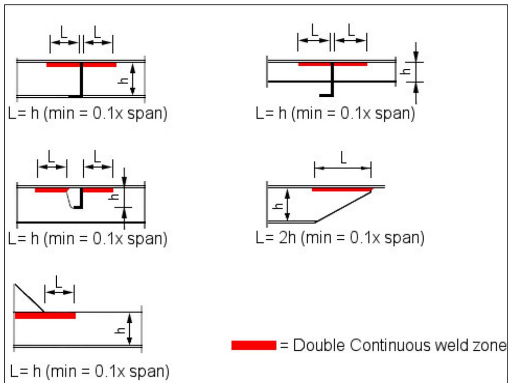
Figure 1: Example stiffening members required double continuous weld zones
