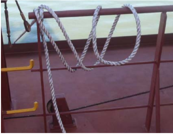
Unapproved secondary means of support tied to non-loading bearing part of accommodation ladder and vessel structure
