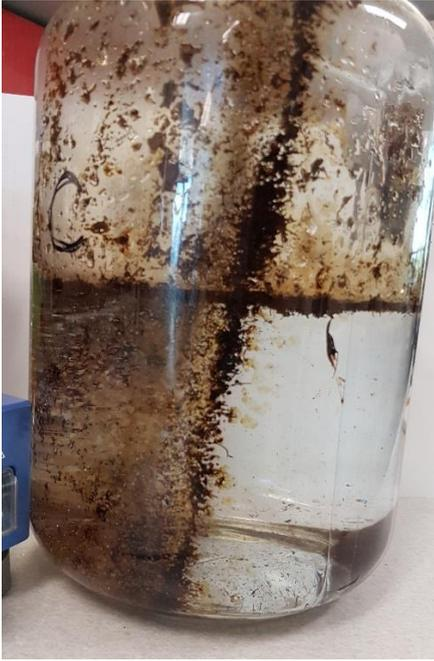
Figure 4: The portion of adsorbent that sank after adding IFO 380
