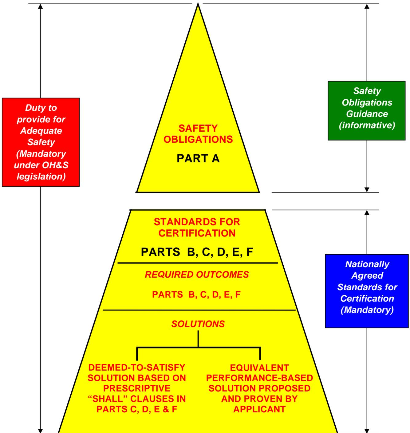
Figure 1 — Structure of the National Standard for Commercial Vessels
