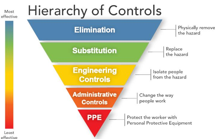
Figure 3: Hierarchy of Controls diagram <sup>[3]</sup>
