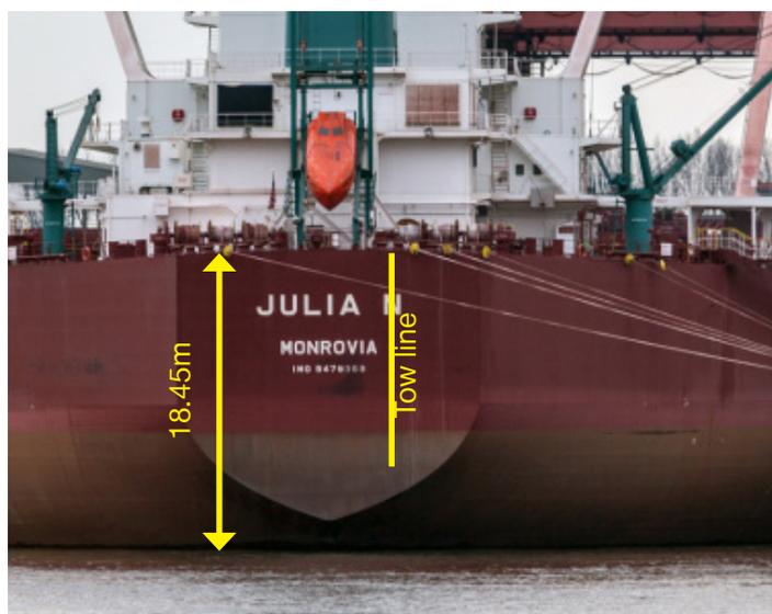
Figure 5: Approximate position of the tow line during retrieval <sup>[1c]</sup>
