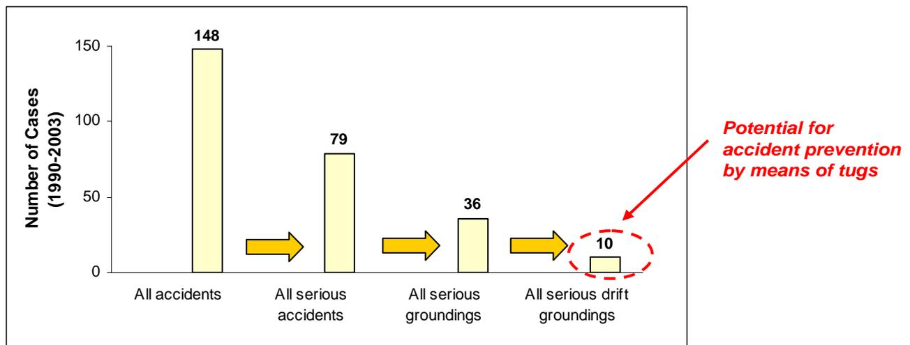
**Figure 5-6 Evaluation of LRFP Accident statistics for Australian waters, 1990-2003**
