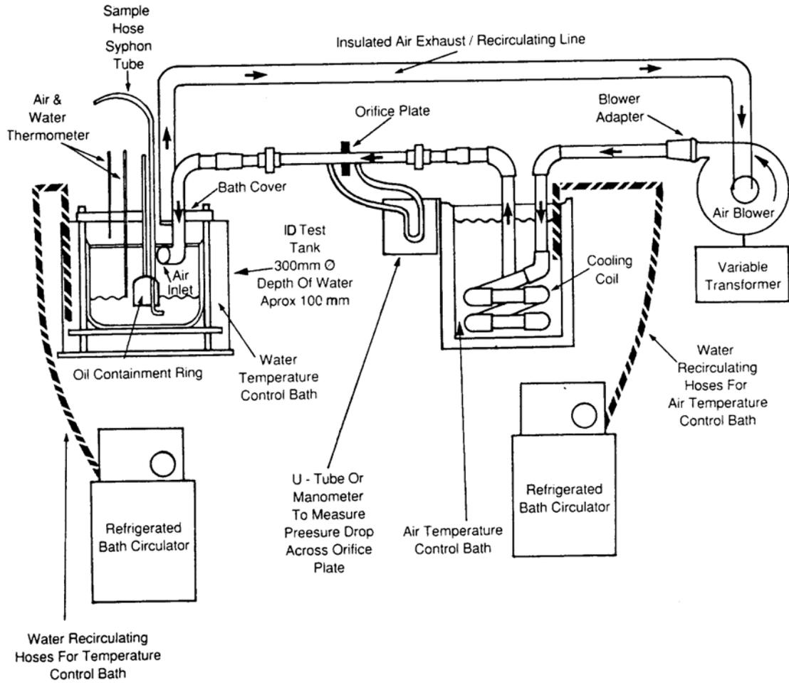
*Figure 2: Mackay (MNS) test apparatus*
