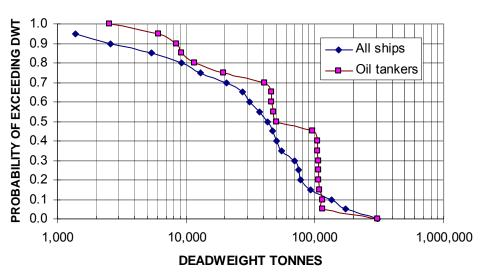
Figure I.3.1 Ship Size Distributions in AUSREP Data
