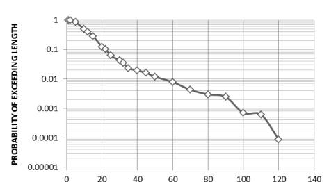
Figure I.4.1 Size Distribution for Small Commercial Vessels
