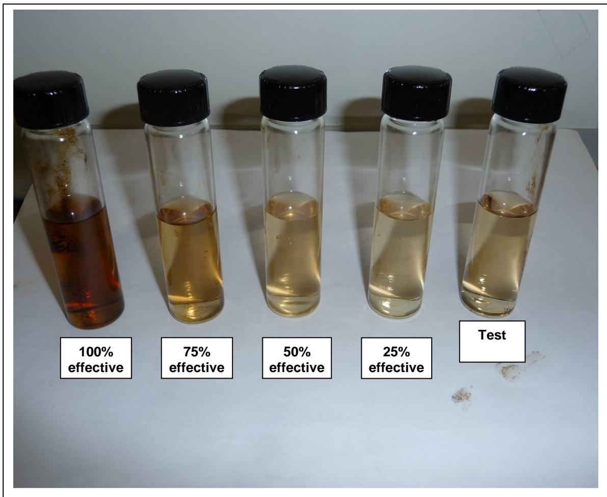
**Step 15 and Interpretation: comparison of test solution (right) and reference solutions (in descending order of effectiveness). The test solution is equivalent to the 50% effectiveness reference solution.**
