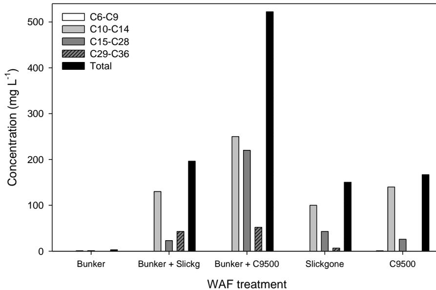
**Figure 3:** Carbon chain length fractionation per treatment and total petroleum hydrocarbon concentration ( $\text{mg L}^{-1}$ ) within the IFO-380, IFO-380 + Slickgone LTSW, IFO-380 + Corexit 9500, Slickgone LTSW alone and Corexit 9500 alone WAF treatments pre-exposure ( $n = 1$ ).
