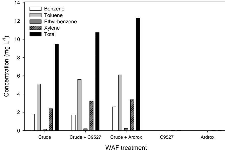
**Figure 2:** BTEX composition ( $\text{mg L}^{-1}$ ) within the crude, crude + Corexit 9527, Crude + Ardrox 6120, Corexit 9527 alone, Ardrox 6120 alone WAF treatments pre-exposure ( $n = 1$ ).
