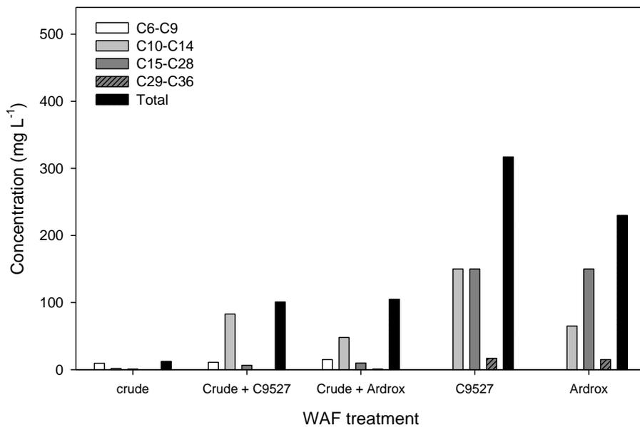
**Figure 1: Carbon chain length fractionation per treatment and total petroleum hydrocarbon concentration (mg L<sup>-1</sup>) within the crude, crude + Corexit 9527, Crude + Ardrox 6120, Corexit 9527 alone, Ardrox 6120 alone WAF treatments pre-exposure ( $n = 1$ ).**
