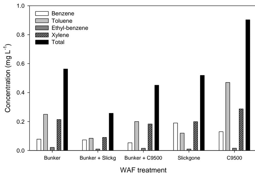
**Figure 4:** BTEX composition ( $\text{mg L}^{-1}$ ) within the IFO-380, IFO-380 + Slickgone LTSW, IFO-380 + Corexit 9500, Slickgone LTSW alone and Corexit 9500 alone WAF treatments pre-exposure ( $n = 1$ ).
