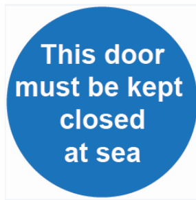
Figure 4 Example of an IMO Mandatory Action Sign for watertight doors
