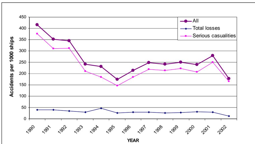
**Figure 5-7 Accident trend for all ship types, serious accidents pr 1000 ships, 1990-2002**
