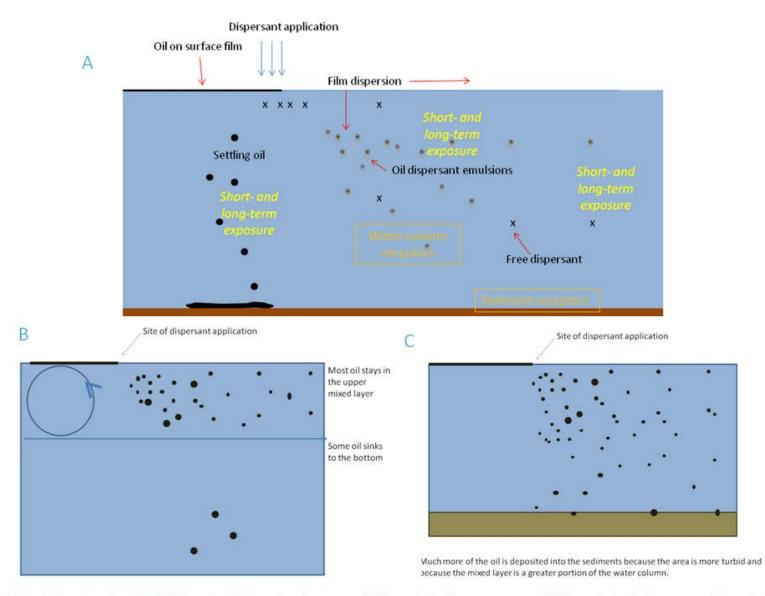
Figure 1. Conceptual model of oil dispersion. A. Overview of processes, B. Dispersion in the open ocean and C. Dispersion in shallower near-shore waters.
