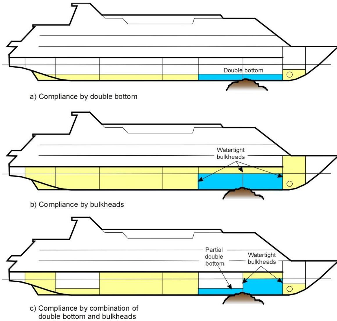
**Figure 3 — Options for control of bottom damage**
