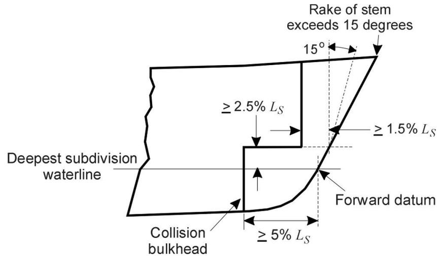
**Figure 8 — Requirements for steps in collision bulkheads**
