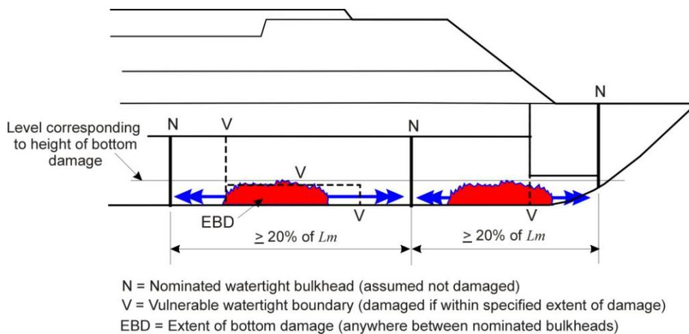
**Figure 4 — Illustration of one-compartment standard (20% min.)**
