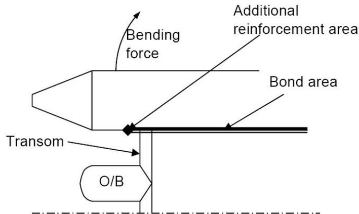
**Figure 14 — Reinforcement in way of an overhanging collar****10.6.4 Fittings for inflation and deflation**
