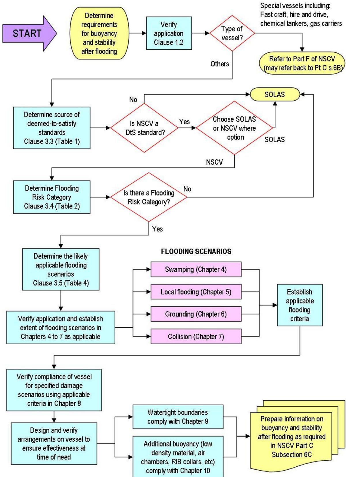
Figure 1 — Flowchart illustrating the use of Subsection 6B
