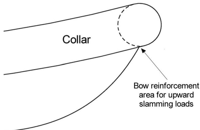
**Figure 13 — Reinforcement at bow**
