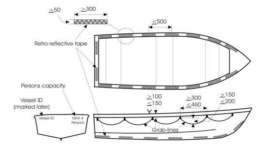
Figure C.1——Dinghy marking and grab-lines
