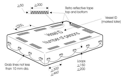
Figure F.1—Buoyant appliance marking and grab-lines
