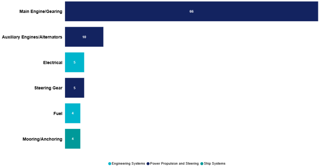
Figure 29: Top 6 technical occurrence type sub-element failures categorised as very serious/serious, FF and RAV 2025
