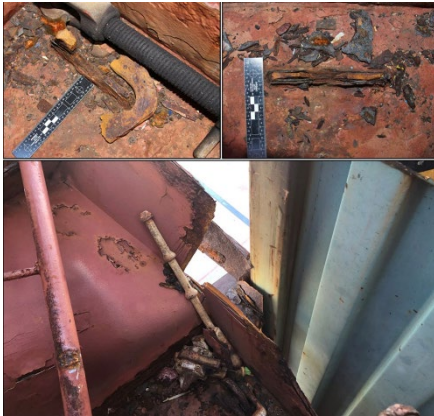
Figure 1: Thinned, heavily wasted and failed lashing eyes (top) and wasted and failed container support structure (bottom) 2
