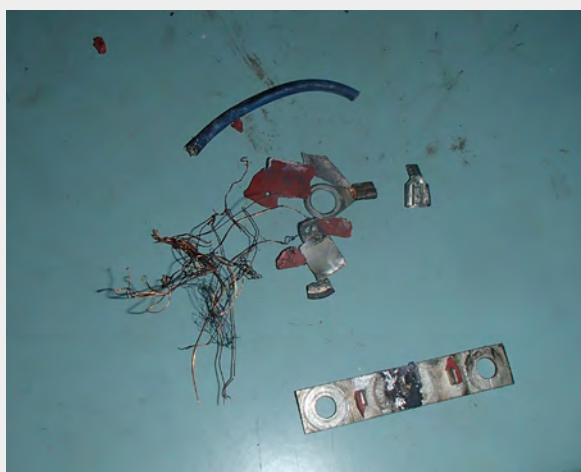
Figure 1: Components ejected from alternator (part of the generator) when tested
