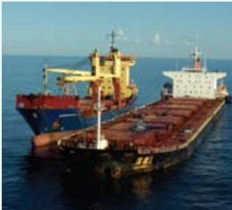
Professional salvors (Svitzer Salvage) were engaged and boarded the *Shen Neng 1* on the morning of 4 April to begin the process of refloating the grounded ship. The initial damage report showed that the main engine room was breached, and the main engine and rudder were both damaged. The action of the sea was causing the ship to move on the reef, creating further damage and increasing the risk of break-up.
