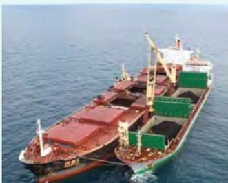
Following the successful internal transfer, large 200-metre lengths of containment boom were placed adjacent to the grounded *Shen Neng 1*, as an important pollution prevention measure before oil could be pumped off the ship. In the prevailing weather, external oil transfer was a difficult and complex operation and the safety of all concerned was of the highest priority.
