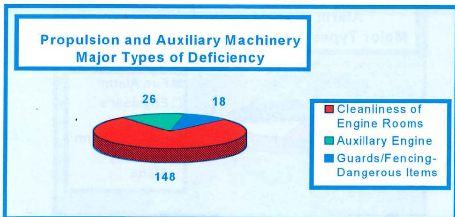
Propulsion and Auxiliary Machinery - Deficiencies
