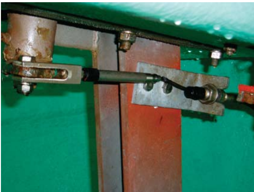
Defective and misaligned operating cable for lifeboat hook release
