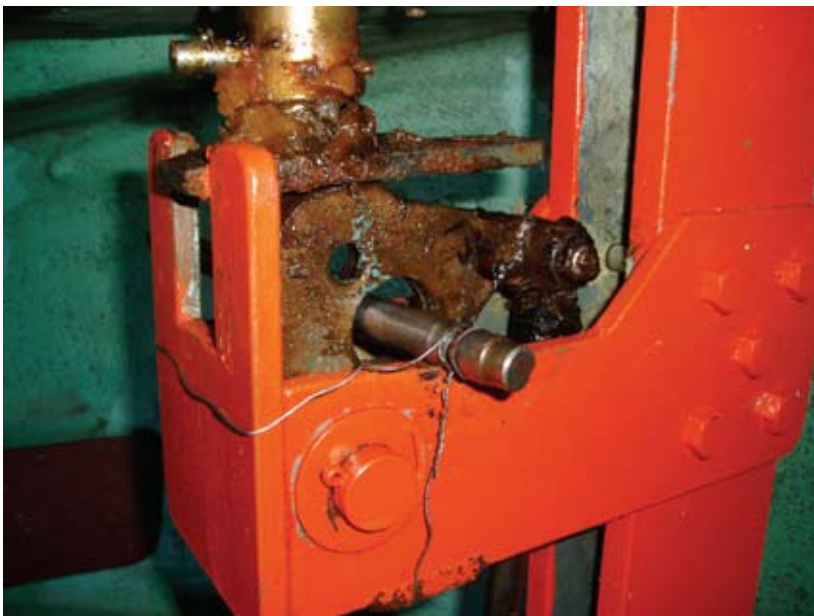
Non reset and overridden lifeboat release
