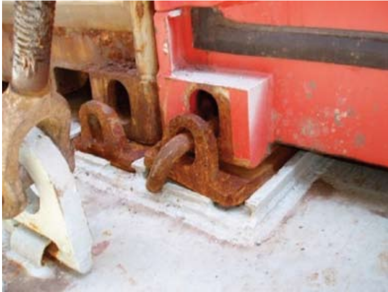
Defective cargo securing arrangement
