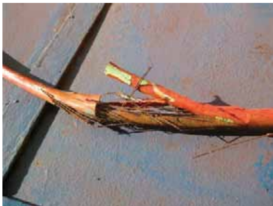
Damaged lifeboat release cable
