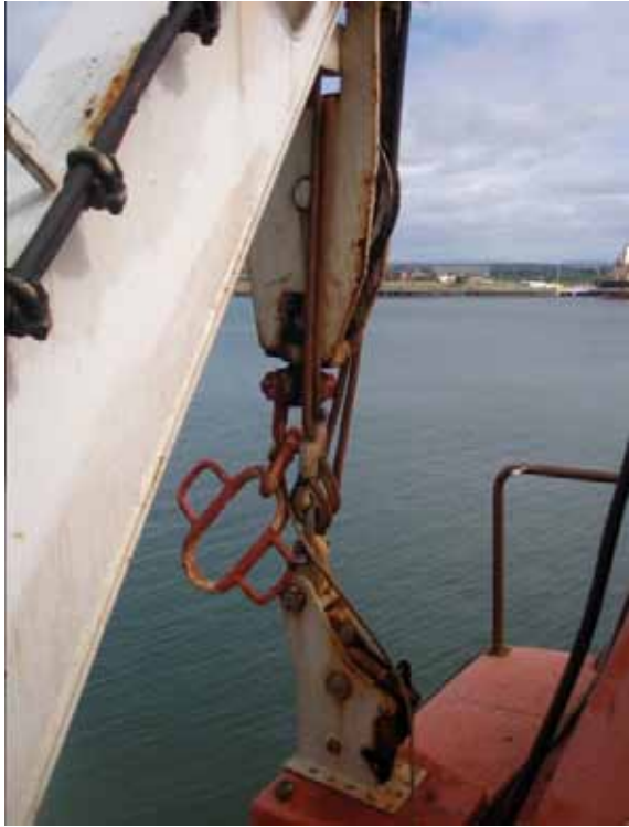
Lifeboat on-load release disconnected
