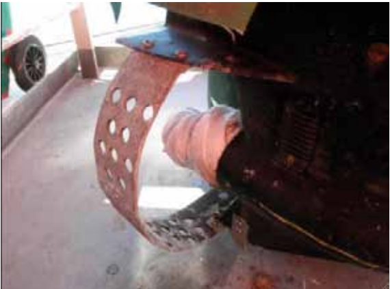
Rescue boat propeller missing
