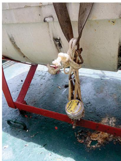
Defective Hydrostatic release
