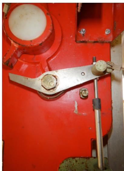
Lifeboat hydrostatic on-load release mechanism locked in open-maintenance position
