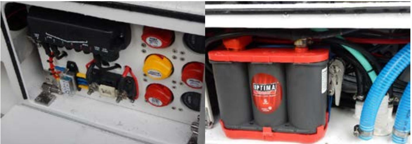
In this example, switch gear and trim tab controls are located within the same compartment as the batteries, causing a risk of explosion. The electrical components were subsequently relocated out of the battery compartment and the batteries were placed into battery boxes. The transom area has since been redesigned by this manufacturer to provide a dedicated battery compartment, removing the source of ignition (engine wiring) from the battery.
