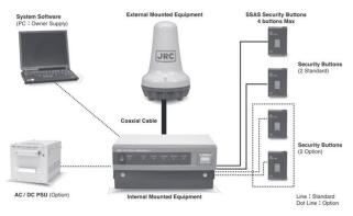
Figure 12 — Typical Inmarsat–C system
