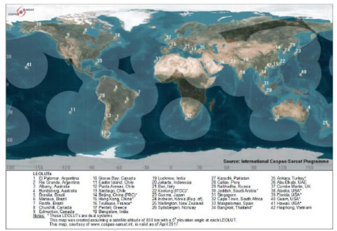
Figure 20 — 406 MHz LEOSAR Satellite Coverage and LEOLUTs
