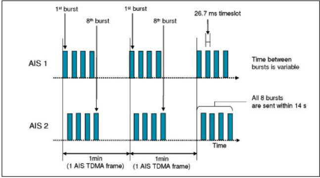
Figure 27 — AIS-SART transmit burst sequence in Active Mode
