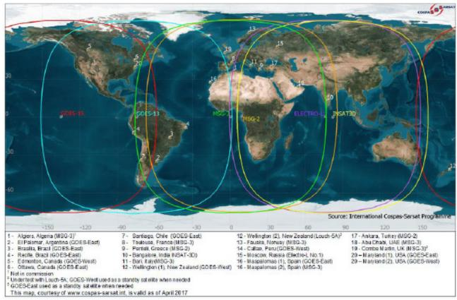
Figure 21 — 406 MHz GEOSAR Satellite Coverage and GEOLUTs
