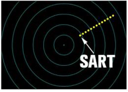
Figure 24 — SART Radar Display
