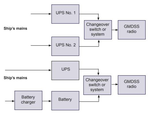
Figure 33 — Typical Uninterruptible Power Supplies
