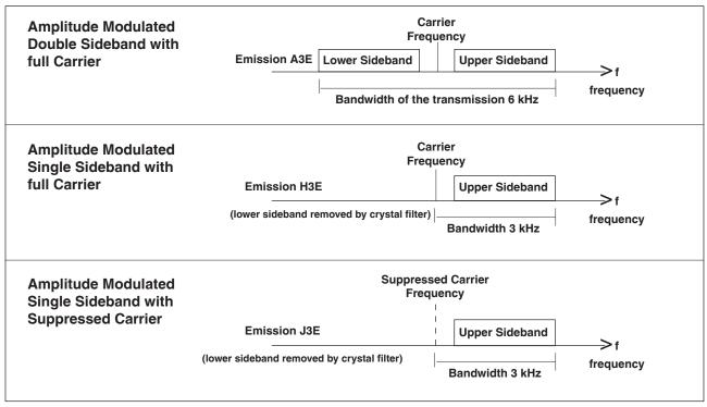
Figure 6 — Various forms of amplitude modulation
