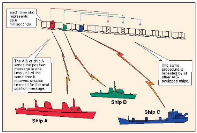
Figure 22 — Principles of SOTDMA
