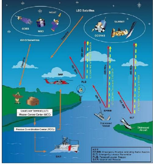
Figure 18 — Basic concept of the Cospas–Sarsat system
