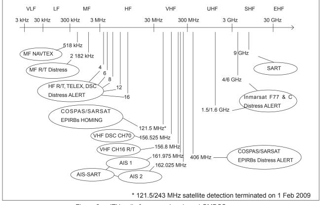
Figure 2 — ITU radio frequency bands and GMDSS usage
