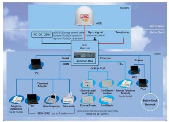
Figure 11 — Typical Inmarsat Fleet 77 installation
