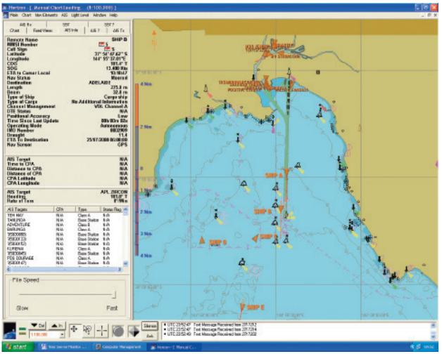
Figure 23 — Screen capture of AIS data
