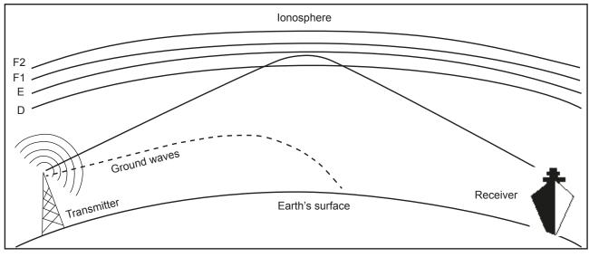
Figure 5 — Propagation of ground waves and sky waves
