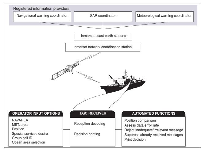
Figure 15 - International SafetyNET Service System Concept
