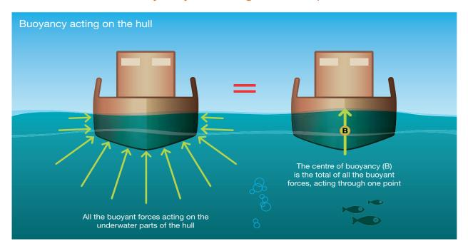
Buoyancy acts on all the underwater parts of the hull. The total of this buoyant upward force can be represented as acting through one point, the centre of buoyancy (B).
