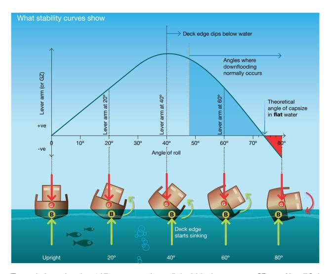
The graph shown above is a stability curve, sometimes called a righting-lever curve or a GZ curve. You will find some of these for your vessel in your stability book if you have one. The small vessels that sit underneath the graph illustrate the corresponding angles of roll and how the forces acting on the vessel move.
