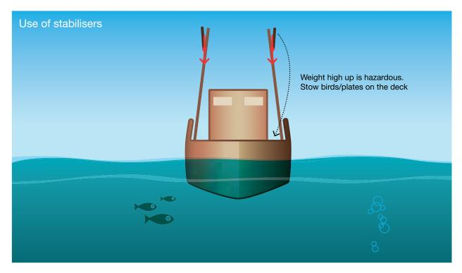
The plates, lifting surfaces or 'birds' must always be stowed on deck while they are not in use. They can weigh more than 100 kg, and leaving them at the top of the arms will significantly reduce a vessel's stability.
