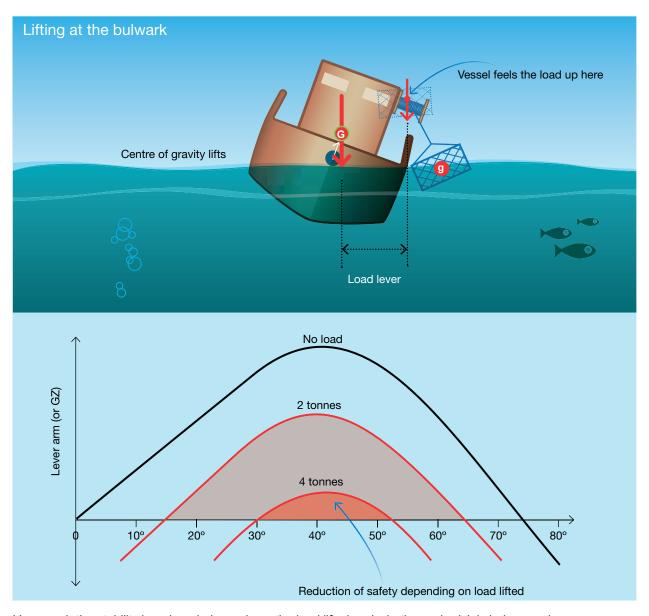
How much the stability is reduced, depends on the load lifted and whether a derrick is being used.
