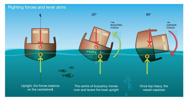
Upright in flat water, the forces at G and B balance each other on the centreline of the vessel.
