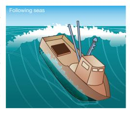
The combination of the next surge of the vessel being off course due to the broaching forces, and the vessel rolling on the next wave face makes a safe course very hard to steer.
