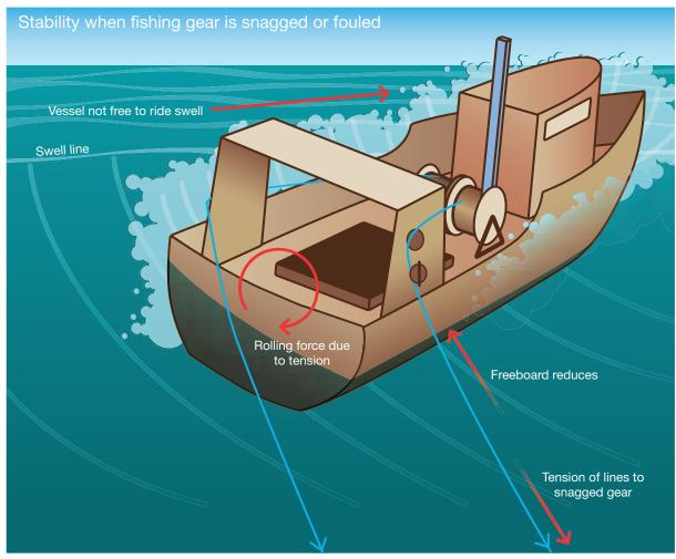
With any gear stuck on the seabed, the vessel is extremely vulnerable:
