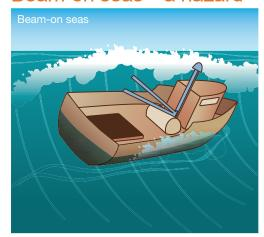
In beam-on seas, there is a high risk of a vessel taking large rolls. If the vessel is also overloaded or subject to another stability hazard, large rolls can lead to capsize.
