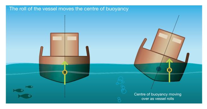
The buoyancy force, acting through the centre of buoyancy (B), moves away from the centreline of the vessel as it rolls over on an angle. The parts of the hull entering the water add buoyant forces on one side, as those parts of the hull on the other side come out of the water. The centre of buoyancy moves to a new position towards one side of the vessel. This is where the buoyancy force will now act.
