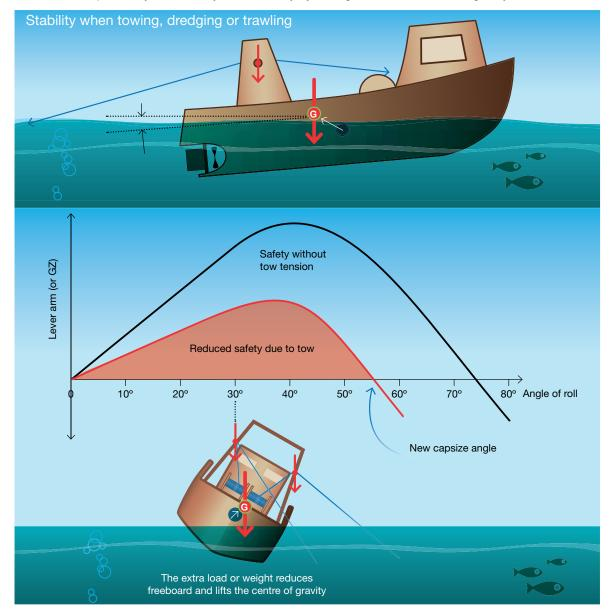
All these factors reduce the stability of the vessel. If the sea-state is rough, or if the vessel is already heavily loaded, the combined effect may be dangerous.
