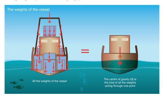
The total weight of the vessel, including all the stores, fuel, equipment and fishing gear, can be represented as acting through one point—the centre of gravity (G).
