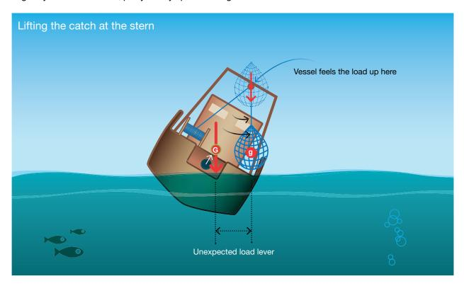
Visualise the gear and full catch at that height—that is how it feels to the vessel.
