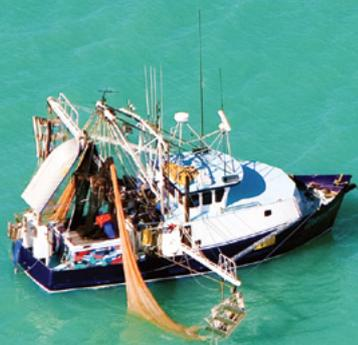
Trawlers can easily roll over and trap crew beneath. The circumstances can differ each time but when a trawler's net gets snagged it is usually a mix of sea conditions, trawler stability and crew actions.
