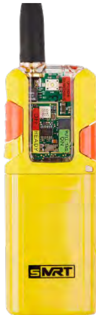
Figure 28 — Maritime survivor locating device (Man Overboard Device) using AIS and VHF DSC
