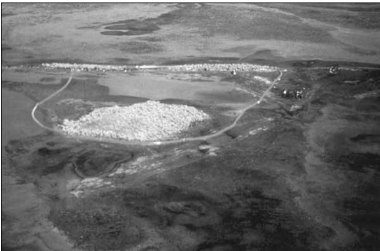
A shore-barrier boom used to protect migratory bird nesting habitats
