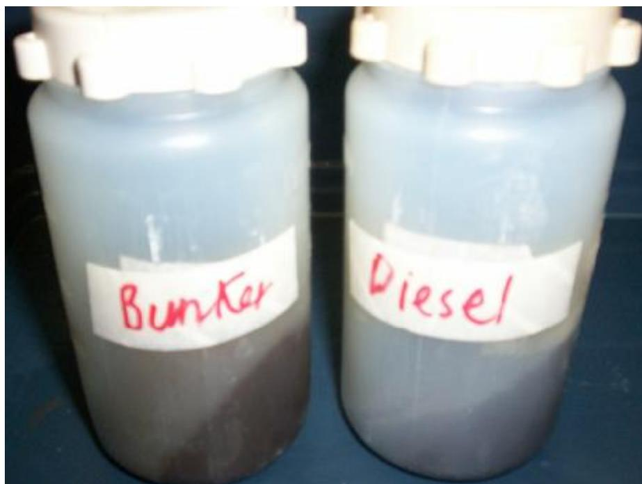
**Figure 65:** Bottles of Diesel Oil and Bunker Oil 1 laden iron powders after centrifugation
