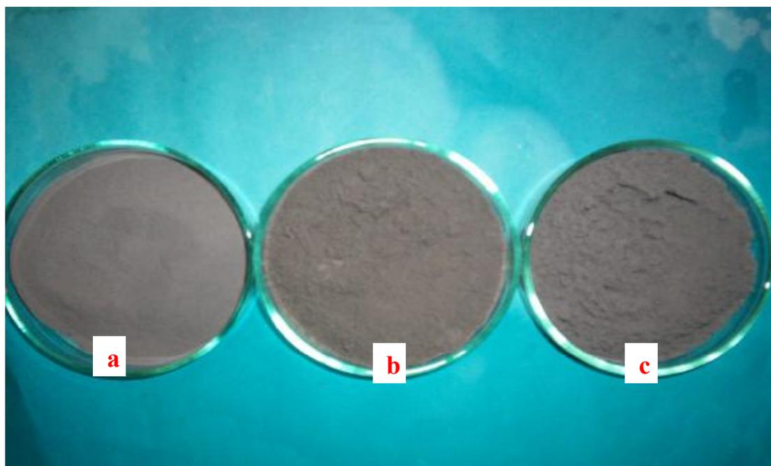
**Figure 66:** (a) Original iron powder; (b) recycled iron powder (from Diesel Oil experiments); (c) recycled iron powder (from Bunker Oil 1 experiments).
