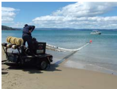
TasPorts employee supervises the rolling out of the rope mop with assistance from the EPA vessel, Liana.
