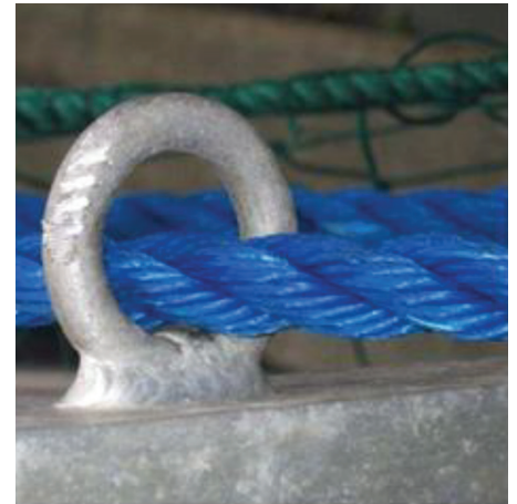
Stanchion eye where the lifting wire got caught
